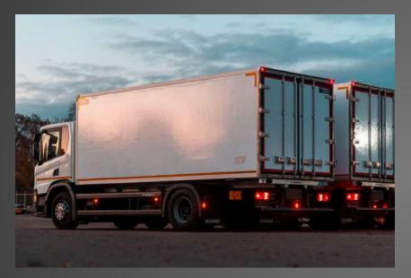
The frameless production technology in collaboration with strong and light sandwich panels made of FRP, water-resistant plywood and extruded polystyrene / polyurethane foam together with structural polymer adhesives and sealants allows the creation of long-lasting and durable truck bodies for various purposes and different needs of the customer.
